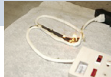
Counterfeiters substitute a 24-gauge wire for 16-gauge wire, creating the risk of a substantial fire hazard.
